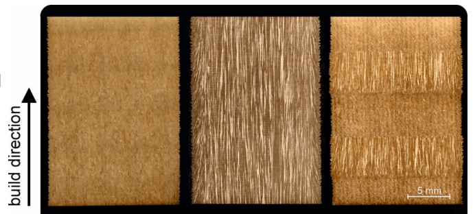
Microstructure control as enabled by EBM Point Melt technology
